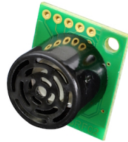
Figure 2.6: SRF02 ultrasonic distance sensor
