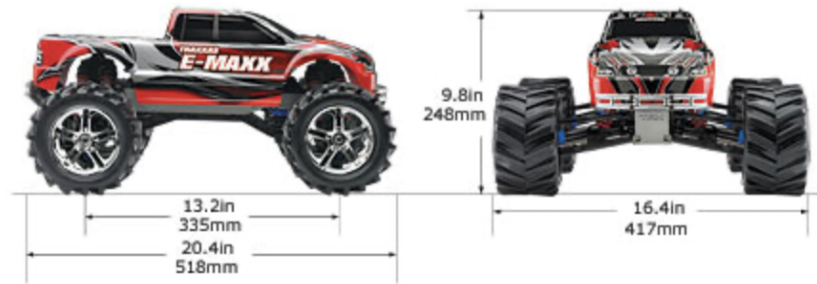
Figure 2.1: Appearance and dimensions of KITT (before modifications)
